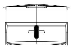
NOTE: The brewing concentration strength increases from left to right using the Strength Control lever.
